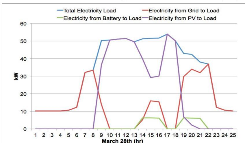
Figure 3. The total electricity load for the Mack Pool on March 28th is met by a combination of energy outputs from the PV, battery (sized to a 6 hour peak) and the remaining pulled from the grid. The PV met approximately 54% of the total load, the battery 4.5% and the grid 41.5%.
